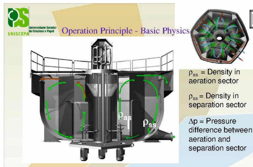
The circulation of stock is based on the difference in the stock's specific gravity between the aeration and separation sectors.
