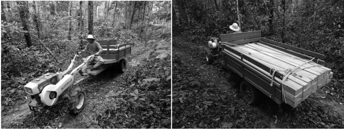
FIGURA 5: Transporte primário da madeira serrada com micro-tractor e reboque. FIGURE5: Transport primary of the lumber with micro-tractor and trailer.
