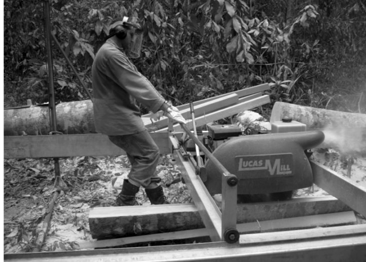
FIGURA 2: Processamento da madeira com serraria portátil. FIGURE2: Processing of wood with portable sawmill.
