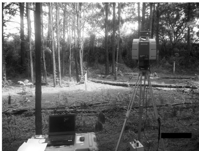
FIGURA 1: Coleta de dados com o equipamento laser HDS3000 no povoamento de pinus. FIGURE 1: Data acquisition with HDS3000 laser equipment in pine stand.
