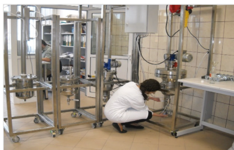
Figure 2. The concept of lignocellulosic biorefinery (on the left) and the lab installation for conversion of raw material from SRWC (willow, poplar, robinia pseudoacacia) to ethanol. [10]
