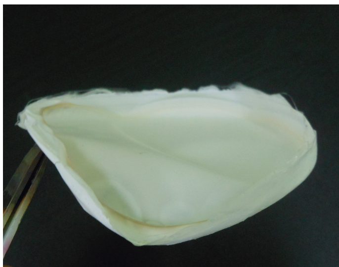
Figure 2. PHBV film extracted from B. xenovorans LB400 culture grown on glycerol waste and valeric acid.
