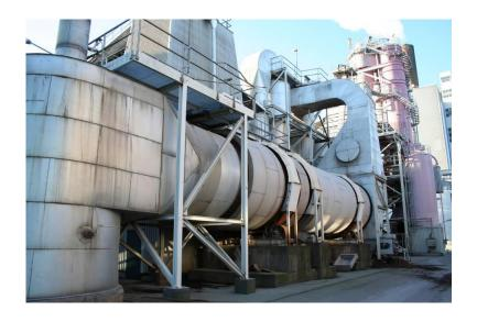
Rotary dryer fired with fuel gas from the gasifier
