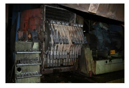
Hammer mills used to produce powder finer than 1 mm
