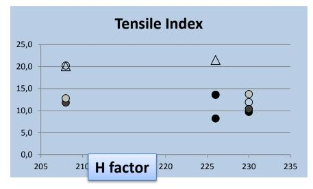
Low severity-low H-factor combinations of SE-Kraft treatments also cause a improvement of bleaching, and maintain mechanical properties (except tear) Refinability experiments are actually been performed o compare the development of properties in SE pulps
